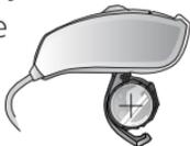
4. Gently close the battery door. If it doesn't close easily, check to see if the battery is upside down.
