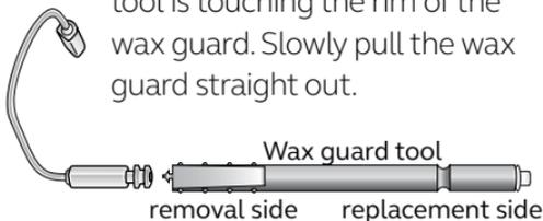
**Insertion:** To insert the new wax guard, gently press the replacement side of the wax guard tool straight into the hole of the sound outlet until the outer ring lies flush with the outside of the receiver. Pull the tool straight out. The new wax guard will remain in place.
